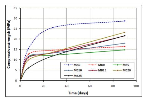
Fig. 6.b- Variation of compressive strength over time
