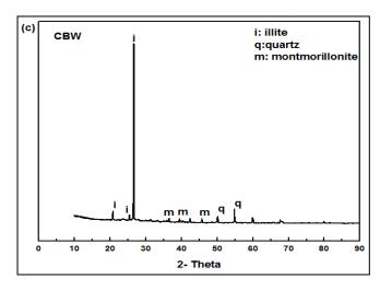
Fig. 2.c- X-ray diffraction patterns of CBW
