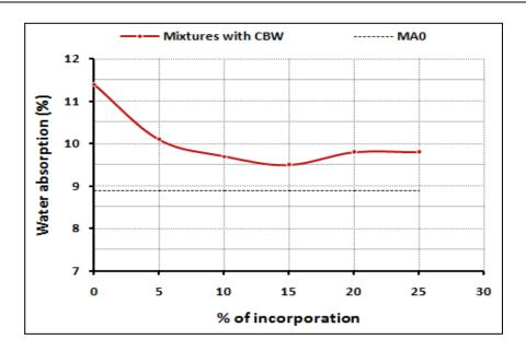
Fig. 8- Effect of CBW amount on water absorption
