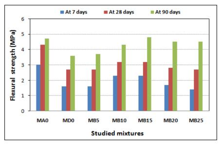
of CBW with incorporation rate of 15%, makes it possible to achieve a flexural strength at 90 days equivalent to that of the control mortar (MA0). This result proved the effectiveness of the used crushed waste.
