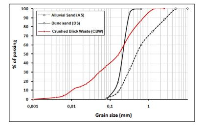
Fig. 1- Particle size distribution of the materials used
