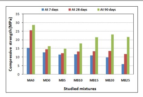
Fig. 6.a- Influence of the incorporation of CBW on compressive strength
