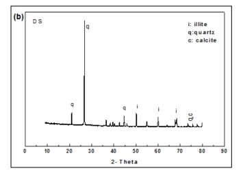
Fig. 2.b- X-ray diffraction patterns of sand DS
