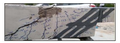
Fig. 10- Cracks Pattern for the Specimen HSTR1-A
