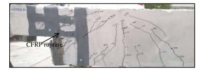
Fig. 14- Cracks Patterns for Strengthening of beam HSTR2-B
