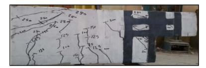
Fig. 11- Cracks Pattern for the Specimen HSTR2-A
