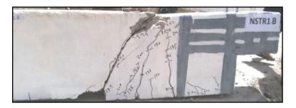
Fig. 19- Crack Patterns for Strengthening beams NSTR1-B
