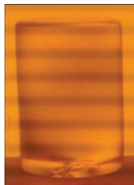
Fig. 3- Visualizations of the model under the polariscope after elimination of the residual stresses for an epoxy cylinder
