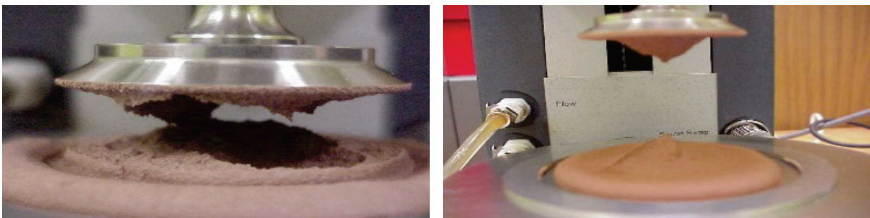
(a) (b) Fig. 9: The rupture profile when increasing polymer concentration
