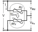
Fig. 3. Equivalent scheme of the studied two-layer structure based on varistor ceramics and PPTC nanocomposite.
