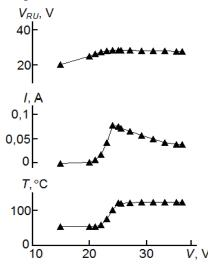
Fig. 2. Dependences of the output voltage  $V_{RU}$ , current *I*, and temperature *T* of the investigated two-layer structure based on varistor ceramics and polymer nanocomposites with carbon filler on the applied input voltage *V*.
