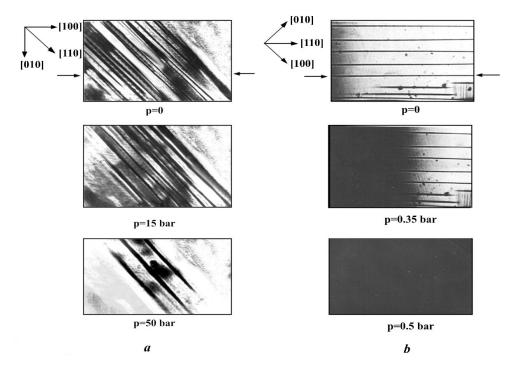
Fig. 1. Formation of single-domain state of NBT crystals: (a) application of axial pressure along [100] direction and (b) along [110] direction near 500 °C.
