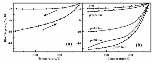
Fig.2. The temperature dependence (a) spontaneous birefringence △n, (b) birefringence at different values of the axial pressure applied along [110] direction of NBT2 samples at heating process.
