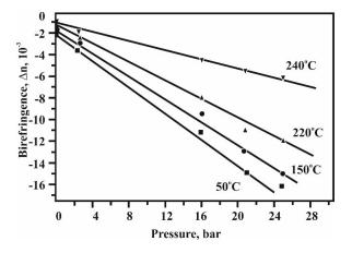
Fig. 3. The effect of the axial pressure applied along [110] direction on birefringence of NBT2 samples.
