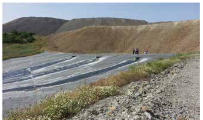
Fig. 4 - 5. The bioleaching of dumps of low-grade copper ores near Radovish, Macedonia
