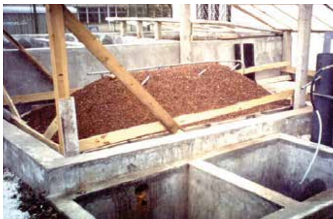
Fig. 8. Pilot-scale operation for microbial pretreatment and leaching of gold-bearing sulphide ores
