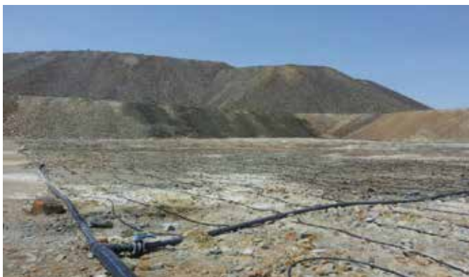
Fig. 4 - 5. The bioleaching of dumps of low-grade copper ores near Radovish, Macedonia
