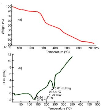
Fig. 3. (a) TGA/DTA and (b) DSC thermogram of the prepared chitosan
