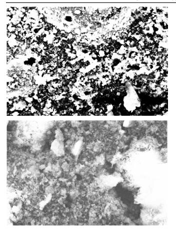
Fig. 4. SEM micrograph of Gel-2 (a) before sorption, (b) after sorption of acephate
