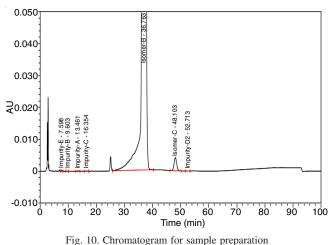
known impurities peaks, purity angles are fewer than the purity threshold. The degradation products of everolimus were effectively separated by the developed method. Hence, the method is considered to be extremely selective and specific for future use. The findings are presented in Table-5.
