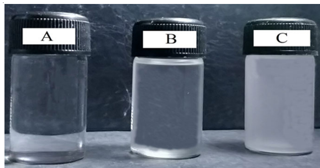
Fig. 3. W/O emulsion representing A: Optically transparent microemulsion; B: slightly turbid emulsion; and C: milky appearance-emulsion obtained by different ratio of Aqueous phase : SPAN 85 : n -decane
