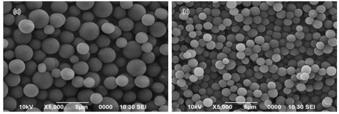
Fig. 2. SEM of NIP (a) and MIP (b)
