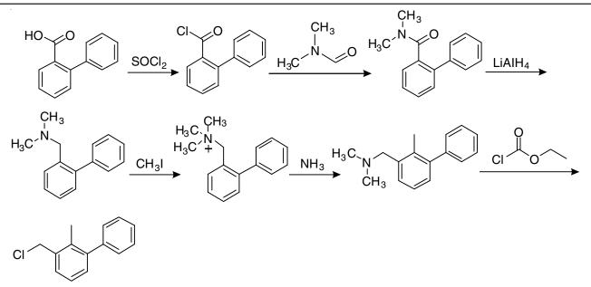
Scheme-I: Traditional synthetic process of 3-(chloromethyl)-2-methyl-1,1'-biphenyl from [1,1'-biphenyl]-2-carboxylic acid
