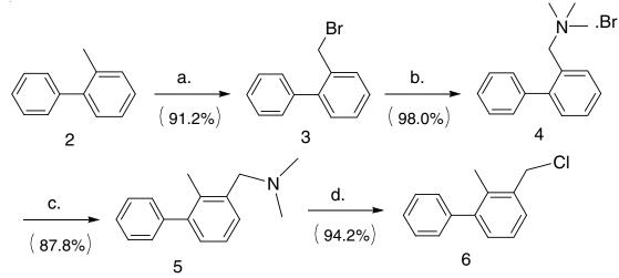
(a) NBS, TBHP, C<sub>6</sub>H<sub>6</sub> (b) N(CH<sub>3</sub>)<sub>3</sub>, ethyl acetate (c) NaNH<sub>2</sub>, NH<sub>3</sub>(l), NH<sub>4</sub>Cl (d) ClCOOC<sub>2</sub>H<sub>5</sub>, C<sub>6</sub>H<sub>6</sub> **Scheme-II:** Synthetic scheme of 3-(chloromethyl)-2-methyl-1,1'-biphenyl from 2-methyl-1,1'-biphenyl
