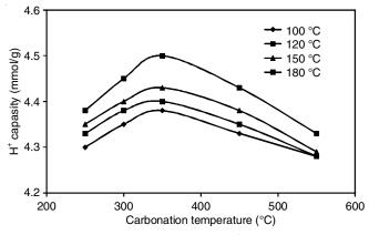
Fig. 3. Effect of carbonization temperature on H<sup>+</sup> activity of sulfonate group (SO<sub>3</sub>H) of the catalyst at various sulfonation temperature
