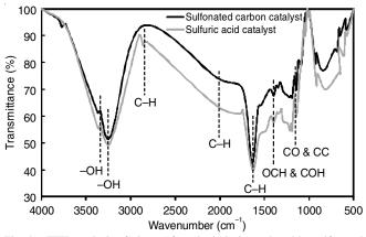
Fig. 4. FTIR analysis of glucose from hydrolysis catalyzed by sulfonated carbon and sulfuric acid
