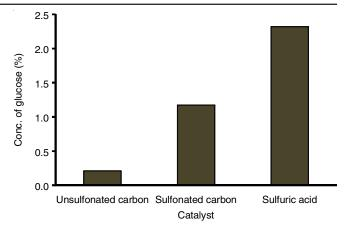
Fig. 5. Concentration of glucose obtained from hydrolysis using three types of catalysts: unsulfonated carbon, sulfonated carbon, and sulfuric acid
