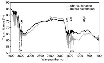
Fig. 2. FTIR of candlenut shell carbon before and after sulfonation
