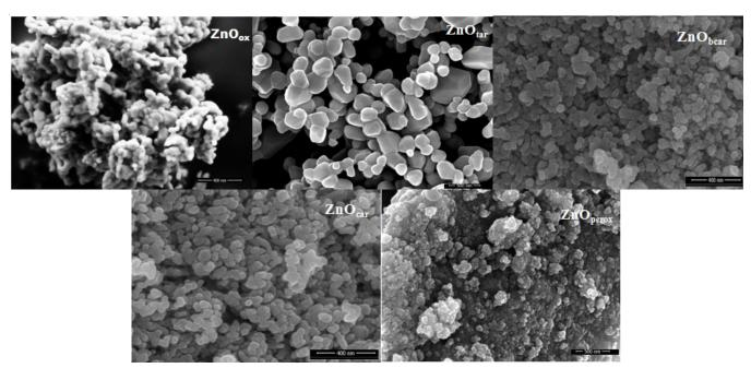
Fig. 5. SEM images of ZnO photocatalysts
