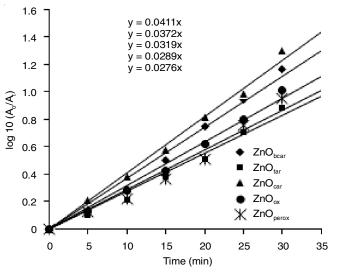
Fig. 7. Kinetics of the decolorization of crystal violet dye in sunlight
