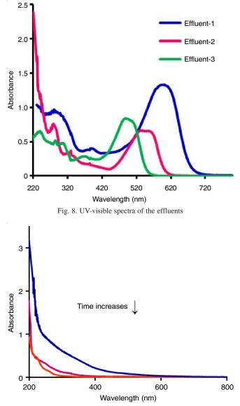
Fig. 9. Absorbance spectra effluent-3 at 60 (decolorization stage), 120 and 180 min time of irradiation
