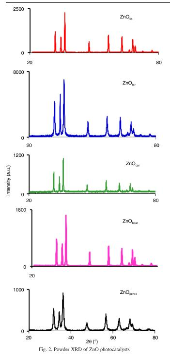
peaks representative of their high crystalline nature. The peaks in XRD can be indexed to the plans [100], [002], [101], [102], [110], [103], [200], [112] and [201] of ZnO crystal. All the photocatalyst showed peak positions at similar diffraction angle
