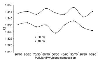
Fig. 6. Plots of RI with composition of 2 % w/v of pullulan/PVA blends at 30 and 40  $^{\circ}\mathrm{C}$
