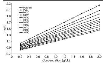
Fig. 1. Plot of  $\eta$  sp/c versus concentration for 2 % w/v, pullulan/PVA blends at 30 °C
