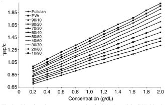
Fig. 2. Plot of  $\eta sp/c$  versus concentration for 2% w/v, pullulan/PVA blends at 40  $^\circ C$
