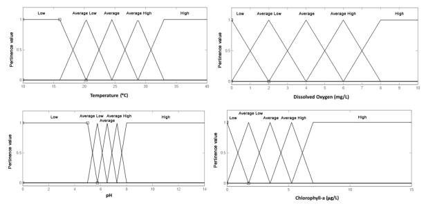
**Figure 4.** Example of fuzzy sets of water quality index for the variables water temperature, dissolved oxygen, pH and chlorophyll-*a*.
