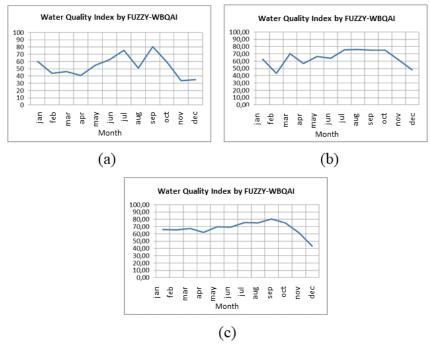
**Figure 8.** Water Quality Index by FUZZY-WBQAI using real data – sampling locations L2 (a), L3(b) e L4(c) (Final index's behaviour).
