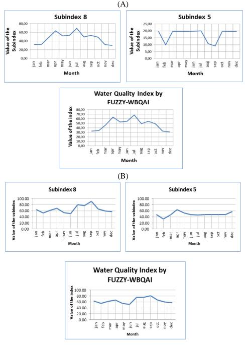
**Figure 7.** Water Quality Index by FUZZY-WBQAI using real data – sampling location L1 (a) and sampling location L5 (b) - Final index's behaviour.
