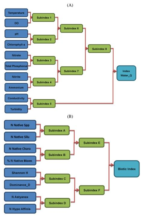
**Figure 3.** a) Flowchart of the sub-indices that compose the Water Quality Index; b) Flowchart of the sub-indices that compose the Biotic Quality Index.
