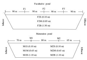
**Figure 1.** Sampling points in the facultative and maturation ponds of module A of the wastewater treatment plant of Trindade, Goiás, central Brazil. S: surface; M: middle; B: bottom.
