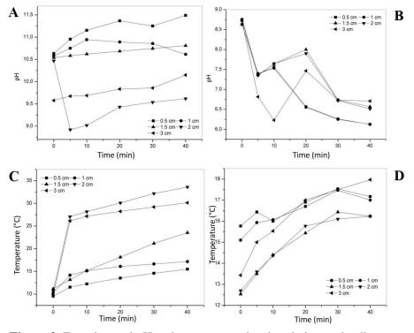
**Figure 2.** Experimental pH and temperature data in relation to the distances (0.5, 1, 1.5, 2 and 3 cm) between the electrodes during the electroflocculation process. A and C - using aluminum electrode; B and D - using zinc electrode. Applied potential: 5000 mA.
