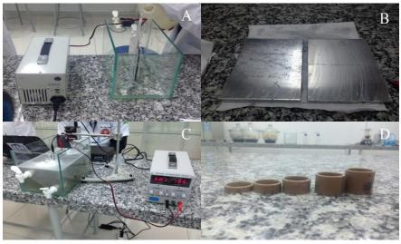
**Figure 1.** (A) Aquarium used; (B) Aluminum and zinc plates; (C) Bench reactor; (D) PVC rings.
