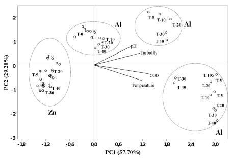
**Figure 4.** Principal component analysis (PCA) for treatment times and parameters evaluated during the electroflocculation process using aluminum and zinc electrodes. T-0 (zero); T-5 (five minutes); T-10 (ten minutes); T-20 (twenty minutes); T-30 (thirty minutes) and T-40 (forty minutes). Al (aluminum electrode); Zn (zinc electrode).
