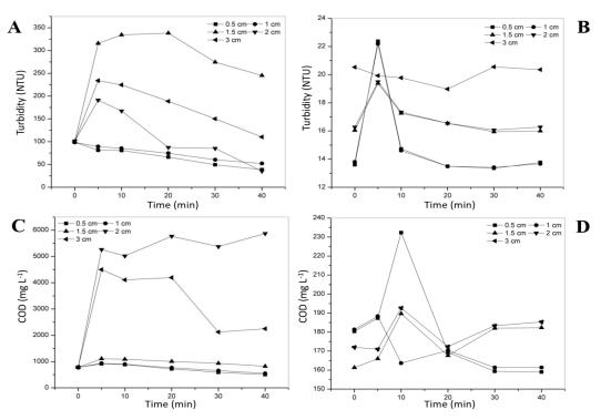
**Figure 3.** Experimental turbidity and COD data in relation to the distances (0.5, 1, 1.5, 2 and 3 cm) between the electrodes during the electroflocculation process. A and C - using an aluminum electrode; B and D - using a zinc electrode. Applied potential: 5000 mA.COD analysis studies the quality of dissolved oxygen. It is an important parameter in the characterization of polluted water (Bittencourt *et al.*, 2018).
