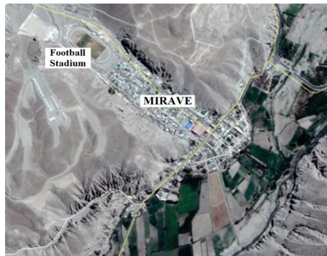
Figure 2. The location of Mirave's population center occupies the entire channel of the outlet mouth of the main stream, and the area of the dejection cone of Mirave's watershed, an area that belongs to the flow path and deposition area of debris flows. Source: Google Earth (2016).
