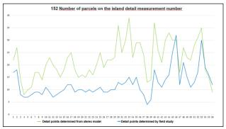
Fig. 12. Detail point comparison on parcel basis.
