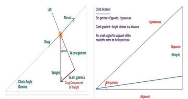
Fig. 6. Opposite = Altitude/Height, Adjacent = Horizontal Distance and Hypotenuse = Slope Distance.
