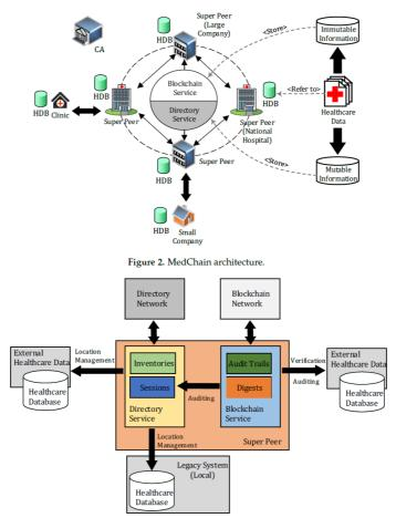
Figure 17. Medchain architecture and its super peer modules (Shen et al., 2019)
