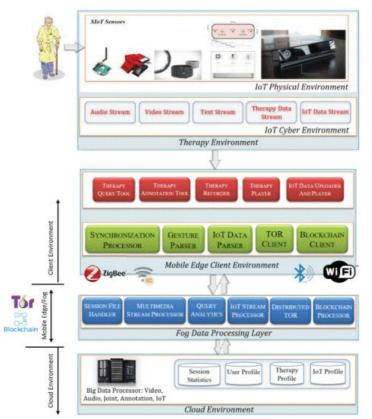
Figure 18. Secure data flow of MEC therapy application through different environments (Rahman et al., 2018)
