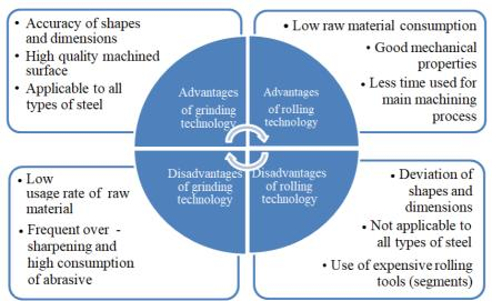
Figure 7. Basic features of SB grooves making technologies
