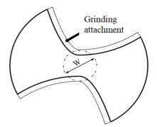
Figure 8. The scheme of SB groove making by a new technological procedure
