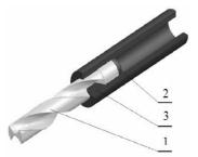
**Figure 5.** Making of SB groove by extrusion: 1 – SB, 2 –material, 3 – matrix (Bulzak & Pater, 2013)
