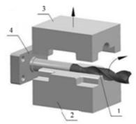
**Figure 6.** Making of a SB groove by extrusion in a two – part mould: 1 – SB, 2 – lower part of the mould,
