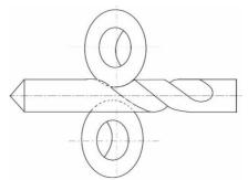
Figure 4. Making of a drill bit groove by rolling technology
