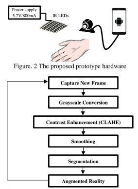
Figure. 3 Real-time vein mapping system diagram
