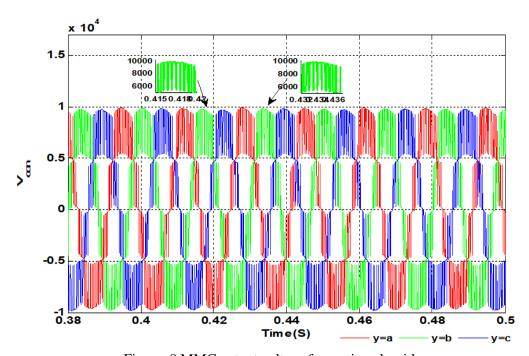
Figure. 8 MMC output voltage for sorting algorithm
