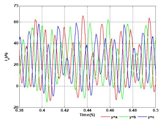
Figure. 7 Circulating current in three legs of converter
