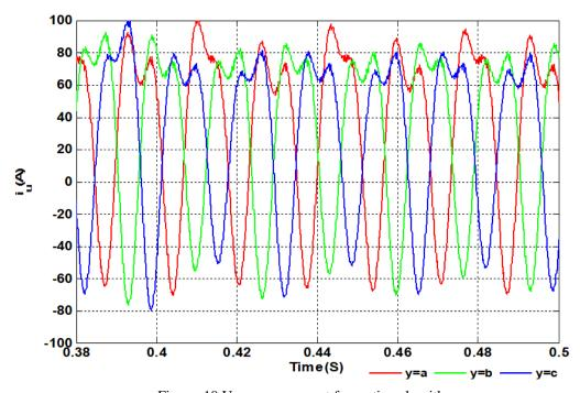
Figure. 10 Upper arm current for sorting algorithm
