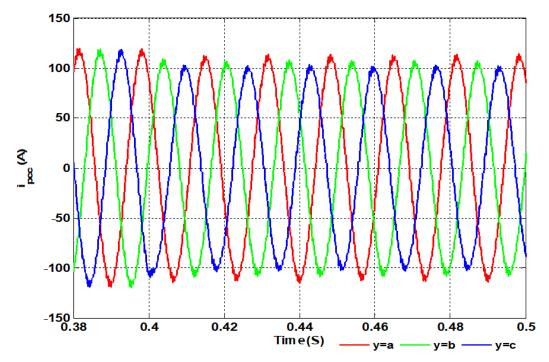
Figure. 5 Current at PCC from converter
