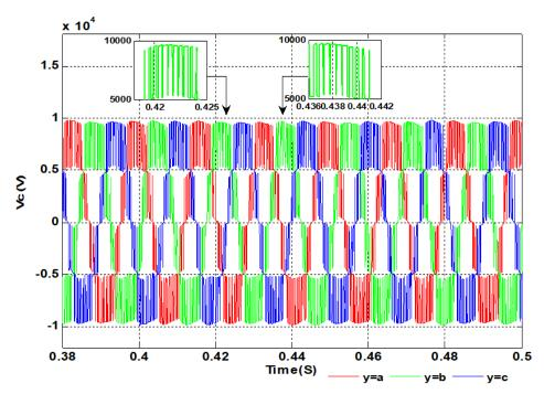
Figure. 4 MMC output voltage
