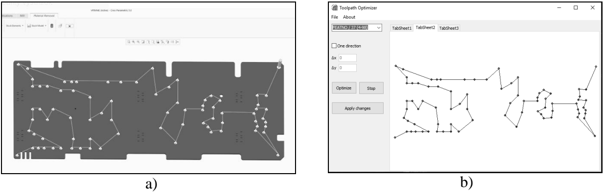
Fig. 4. a) non-optimized tool path of the drilling operation generated by the system Creo b) non-optimized tool path loaded in the application Toolpath Optimizer
