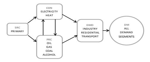
Figure 1. A simplified illustration of main components of a typical RES model (Sulukan, Özkan & Sarı, 2018).
