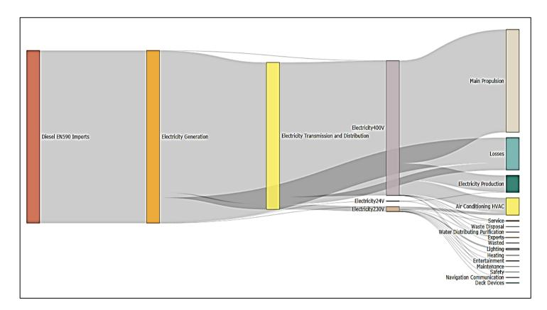
Figure 6. LEAP energy flow (Sankey) diagram of the analyzed ferry.
