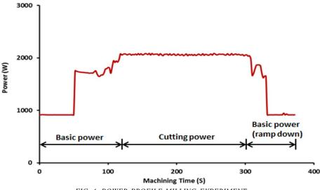
FIG. 4. POWER PROFILE MILLING EXPERIMENT
