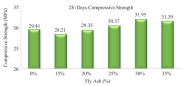
FIG. 3. COMPRESSIVE STRENGTH OF 28-DAYS TEST RESULT WITH INCREASE OF FLY ASH
