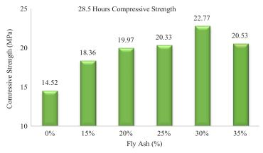
FIG. 2. COMPRESSIVE STRENGTH OF 28.5 HRS TEST RESULT WITH INCREASE OF FLY ASH
