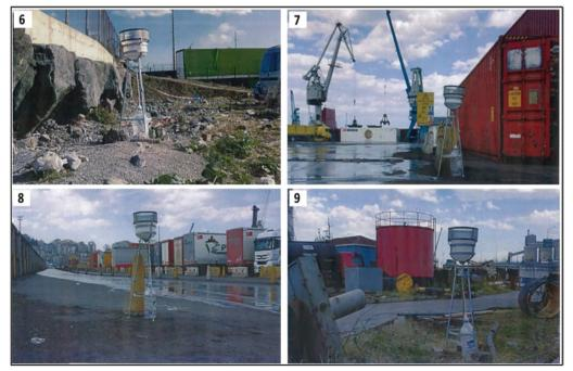
*Figure 5.* PM (deposited dust) Measuring Points, (6) beside Guest Parking Area, (7) front of Dock 3, (8) next to Loading Area 4-5, (9) Bilge Area
