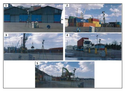
*Figure 4.* PM<sub>10</sub> Measuring Points, (1) Stock Area, (2) Dock 3, (3) Dock 4, (4) beside Weighbridge, (5) Truck Crossing Road
