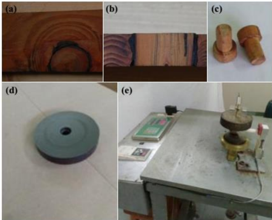
Fig. 1 Experimental pine wood a) top view, b) front view, c) wear sample of wood and knot, d) MS counter disk and e) wear testing machine
