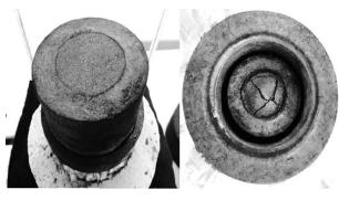
Fig. 4. The matrix filled with a sample of natural graphite: a - before treatment; b - after treatment
