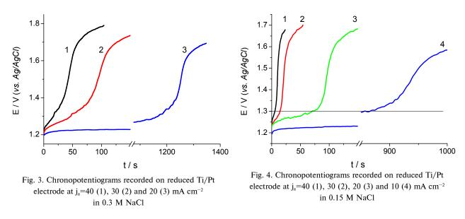
Electrolysis of sodium chloride solutions on Ti/Pt anodes under current reversal conditions
