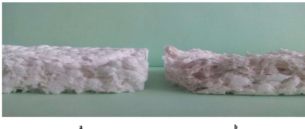
Fig. 4. Photos of the block thermal insulation materials obtained by volume (a) and contact (b) grouting
