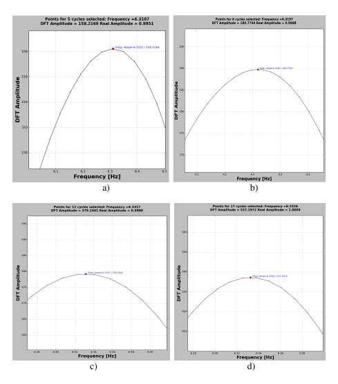
**Figure 2.** The overlapped spectra containing the DFT samples used for interpolation obtained after many signal truncation
