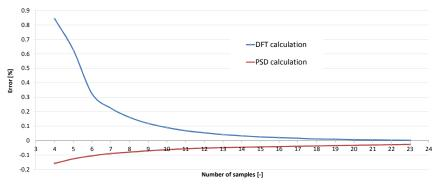
Figure 4. Error curves for interpolation made on DFT respectively PSD samples
