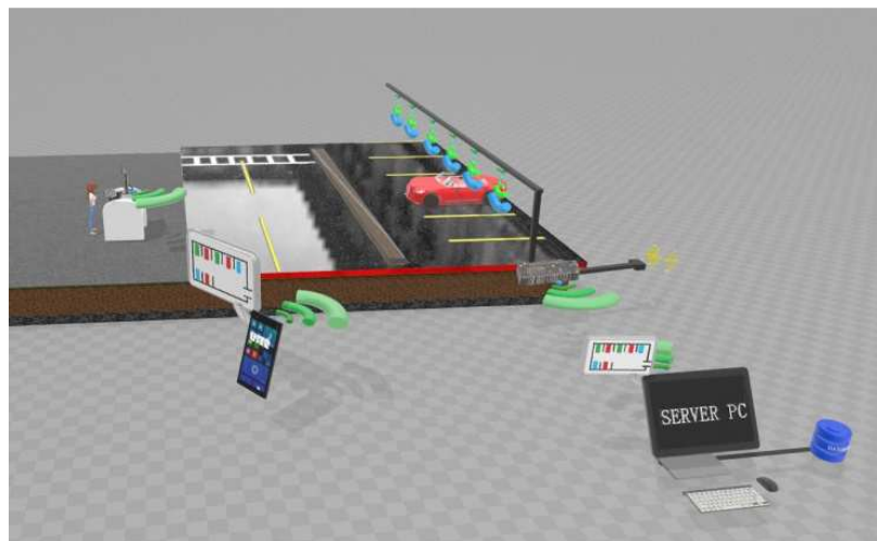
Figure 3: After the User Verifies the Scan Code, the User Gets an Overview Map of that Parking Area According to which the User Parks His Car in the Desired Parking Slot. Once the Car is Parked, this Data is Updates in the Database.
