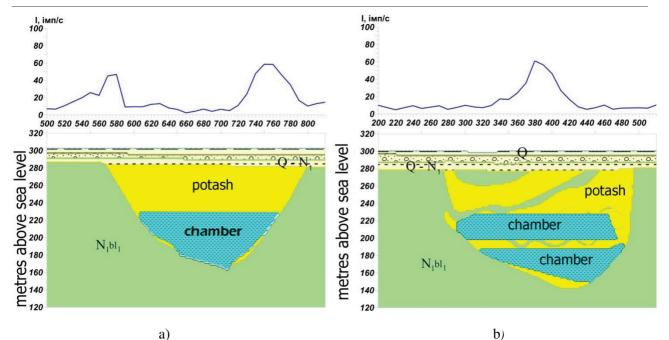
Fig. 4. Geological section and graphics of the ENPEMF
