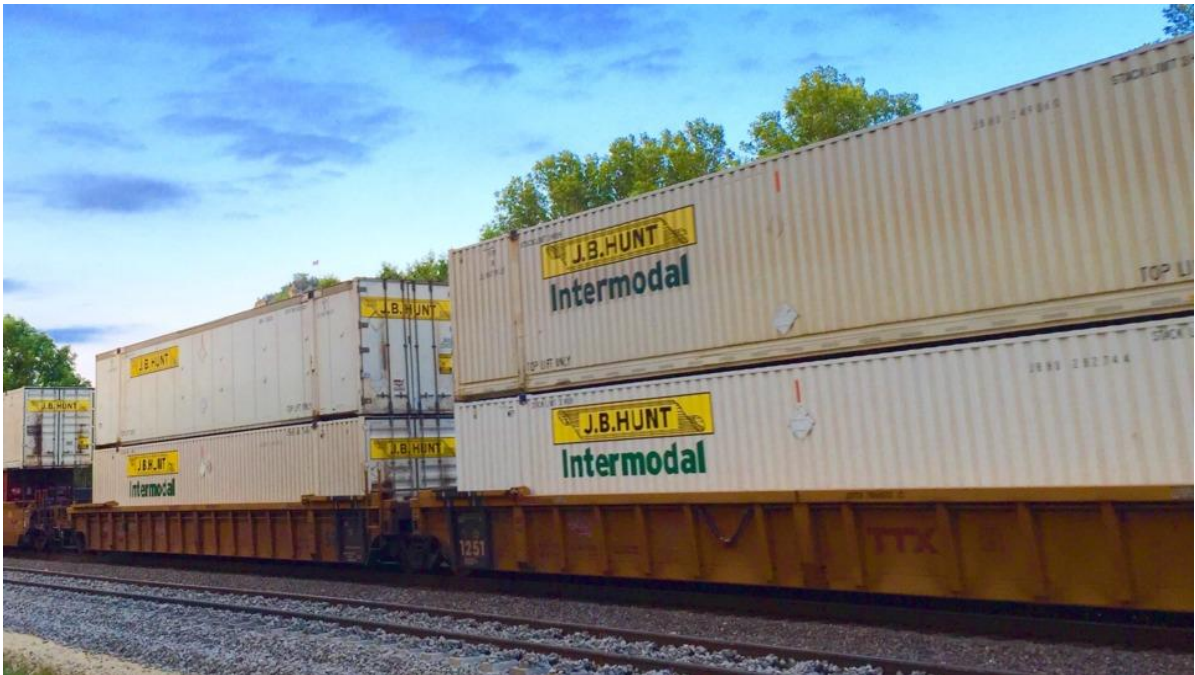
Fig. 10. Transport of containerised cargo using the double-stack system
