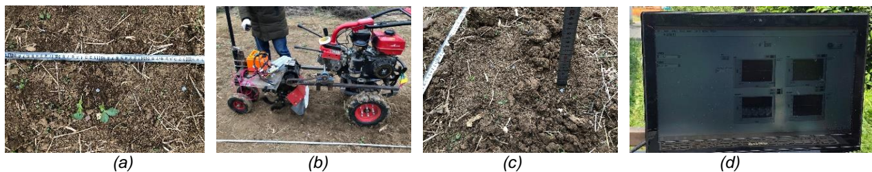
Fig. 6 - Illustration of test procedure (a) Tracer pellets set; (b) Platform; (c) Data measurements; (d) Power consumption collected
