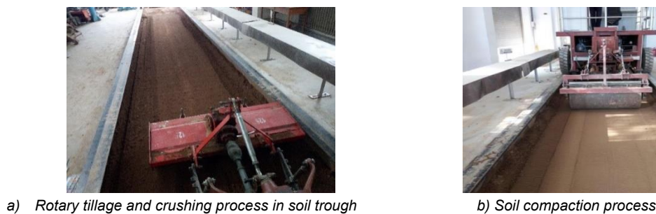
Fig. 2 - The soil preparation process of the soil trough
