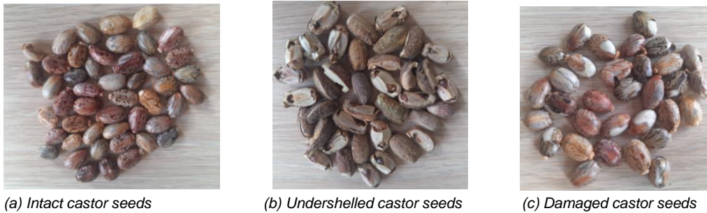
Fig. 10 - Shelling effect of the testbed
