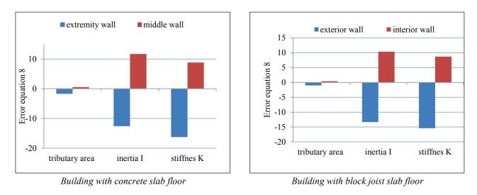
Figure 9- Distribution shear force in walls for building of 3.14:1 aspect ratio assumed rigid and with opening of size 0.64%
