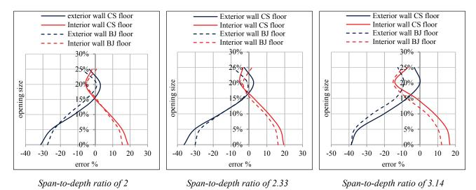
Figure 8 summarizes the error between inertia method and finite element method for all building with position 3 for diaphragm assumed flexible.
