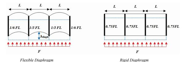
Figure 5- Distribution of Horizontal Forces in the Wall.
