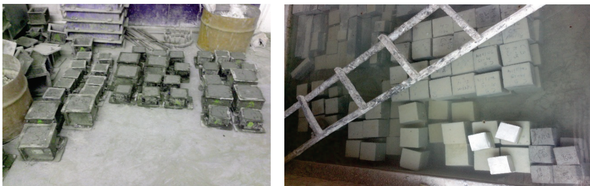
Figure 4- Casting and curing of specimen's
