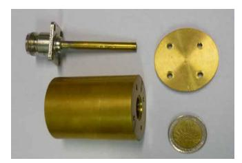
Fig. 13: Utensils used to measure the transmission line in short-circuit.
