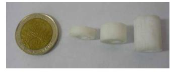
Fig. 14: Teflon slabs of thicknesses d = 4 mm, d = 8 mm and d = 16 mm.
