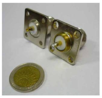
Fig. 12: Adjusted connector and original reference connector.
