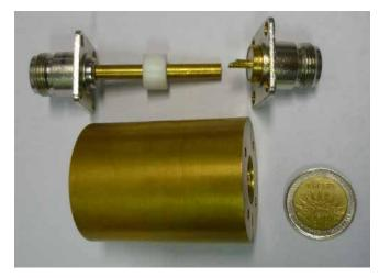
Fig. 11: Sample holder with the inner and outer cylindrical conductor, a Teflon sample with d = 8 mm and two connectors.
