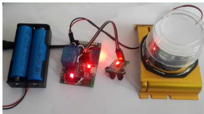
Picture 1 - Dust Sensor with microcontroller.
