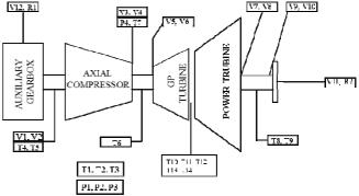
Fig. 1 - Position of embedded sensors on the turbine under consideration.
