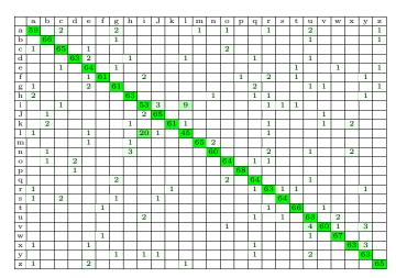
For most letters, the network found a good classification. The letters that were easier for the network were: p (98.5%), w (97.1%), b (95.65%) and t (95.65%). On the other hand, the letters that imposed the greater difficulty were: l (65.21%), i (76.81%), a (85.5%), n (86.95%) and v (86.95%). The main confusions committed by the network were exchanging l by i (28.98%), i by l (13.04%), v by u (5.79%), i by j (4.34%), n by h (4.34%) and v by y (4.34%).
