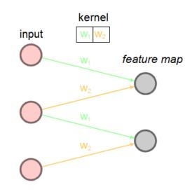
Fig. 3. Neuron weight sharing in the convolutional layer
