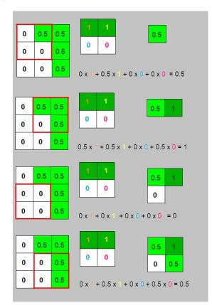
Fig. 4. Example of convolution
