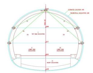
Figure 4. Tunnel deformation survey method
