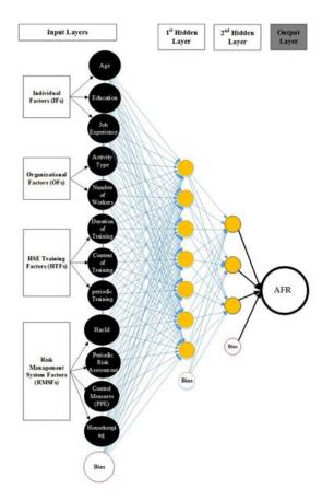
Figure 1: Optimum ANN Structure of AFR in Construction
