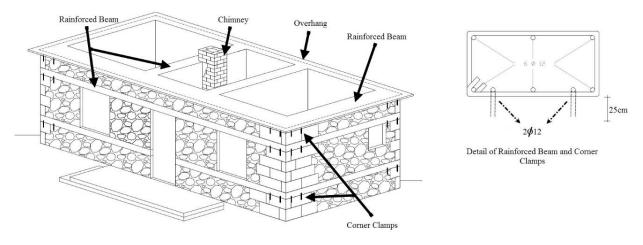
Figure 19: Recommended corner and chimney detail
