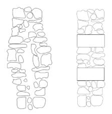
Figure 23: The connection of inner and outer wall layer (Earthquake Regulation 2007)
