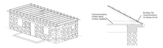
Figure 21: Beam-wall connection and roof details
